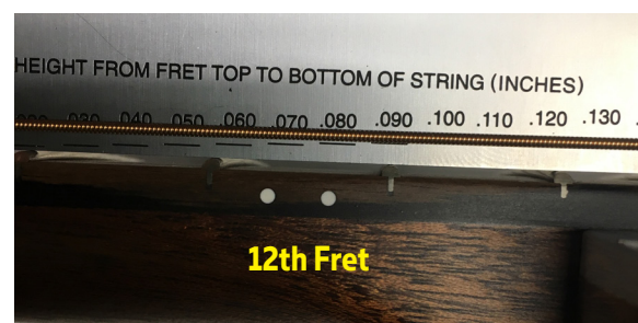
Example showing string action height of .090" at the 12th fret.
