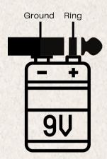
Plug the stereo cord into your instrument. Hold the 9V battery so that the positive terminal is touching the Ring of the stereo plug and the negative terminal is touching the Ground. Hold it like this for 60 seconds and you are ready to play for 16 hours. The system will not be damaged by accidentally connecting the battery in the wrong direction.
